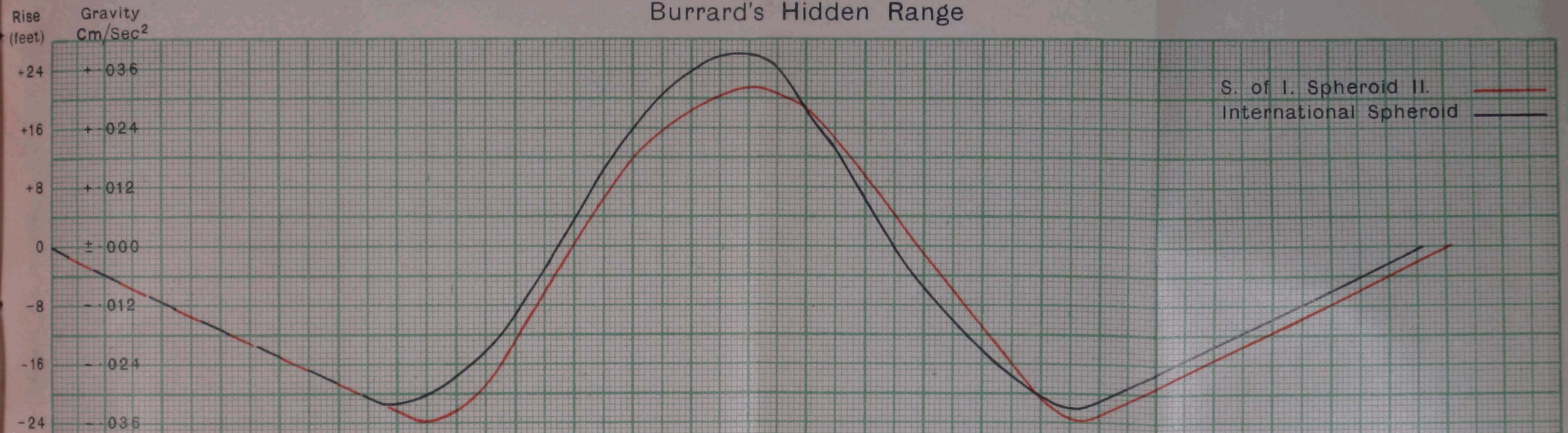
Fig. 2 Burrard's Hidden Range on Section AA Horizontal scale 1 inch=250 miles Vertical scale about 50 times horizontal scale
